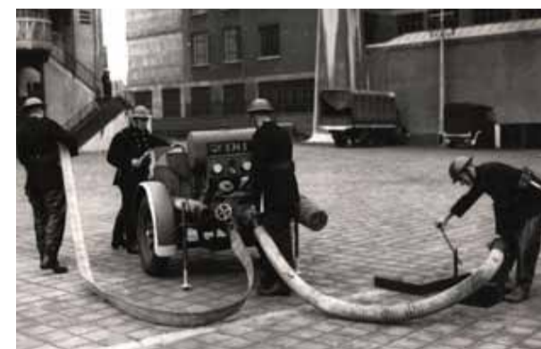
National Fire Service firemen training to use a trailer pump at LFB headquarters, c.1941
